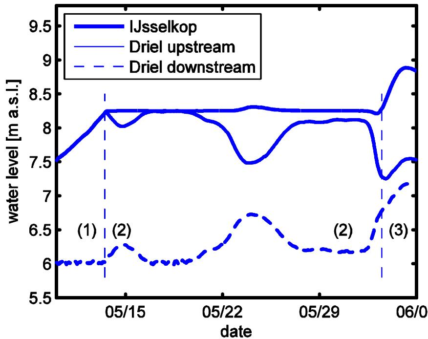
**water level control at Driel during low - medium flow regime in May 2007 with water level set point of 8.25 m a.s.l. at gauge IJsselkop**
