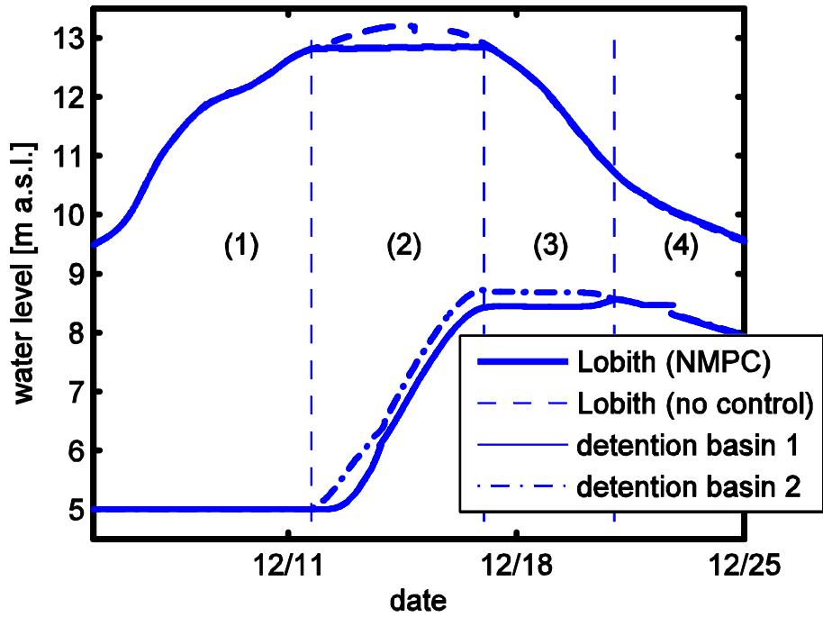
**damping of small flood peak above 12.75 m a.s.l. in December 2007 at gauge Lobith by control of detention basins 1 and 2**
